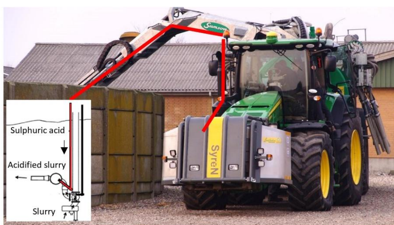
Storage acidification – Slurry acidified in the storage facility during filling of slurry. The final adjustment of the pH may be performed during application to agricultural fields
