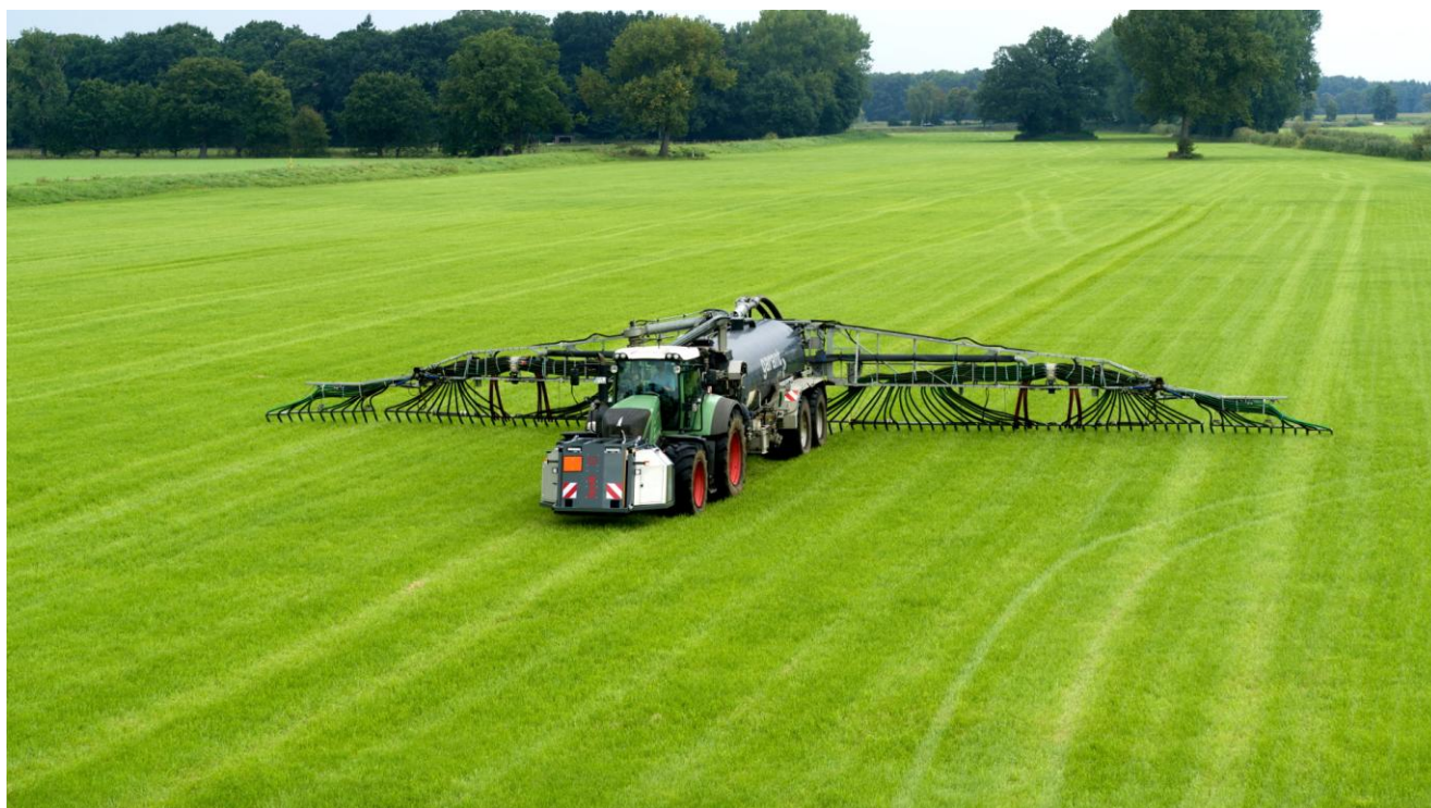
Commercial SyreN process: acid is injected and mixed immediately before the slurry is distributed.
