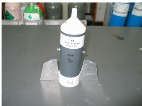
Figure 2. Picture of a passive flux sampler fitted with mounting pivots and fins to keep the device aligned with the wind.
