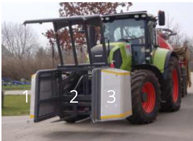
Figure 1. The SyreN technology includes three tanks installed on the front of the tractor. 1: Tank for iron sulphate. 2: Here the tank for sulphuric acid shall be placed. 3: Tank for water for cleaning the system.
