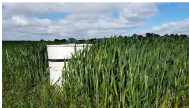
Figure 6. Measurement of nitrous oxide with the use of extensions in wheat by the “closed chamber” technique (Source: Sebastian Neumann, LLUR).
