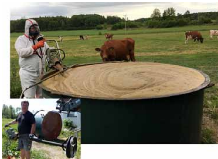
Figure 1. Acidification was performed in a separate tank the day before spreading. An electric driven stirrer was used for mixing acid into slurry. Photo: Marianne Tersmeden
