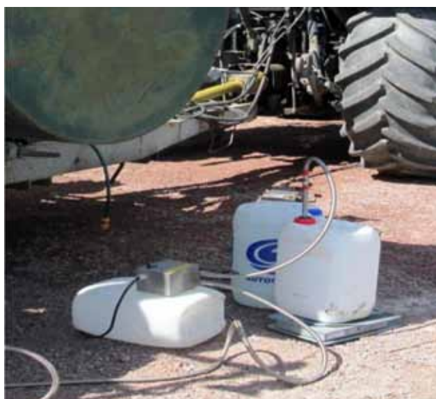
Figure 4. Left picture. The acid container was placed on a scale in order to determine the acid addition and connected to an electric acid pump. Right picture. The acid was pumped through a tube into an iron rod which ended at the recirculation outlet of the spreader pump for mixing the slurry in the tank. Photo: Gunnar Lundin
