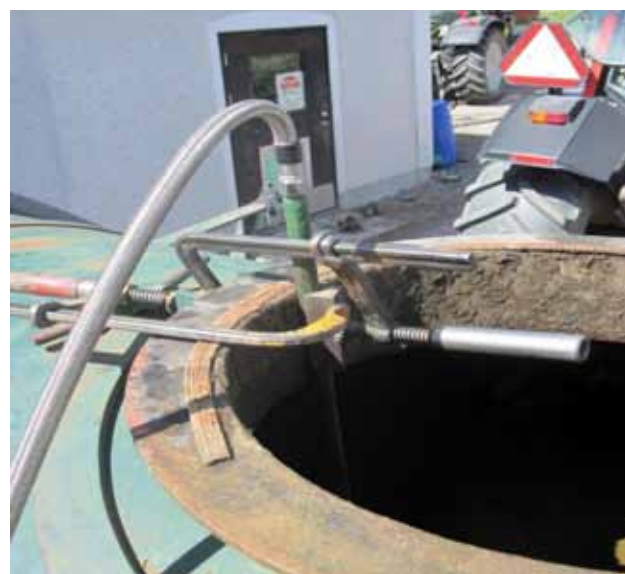
Figure 4. Left picture. The acid container was placed on a scale in order to determine the acid addition and connected to an electric acid pump. Right picture. The acid was pumped through a tube into an iron rod which ended at the recirculation outlet of the spreader pump for mixing the slurry in the tank. Photo: Gunnar Lundin
