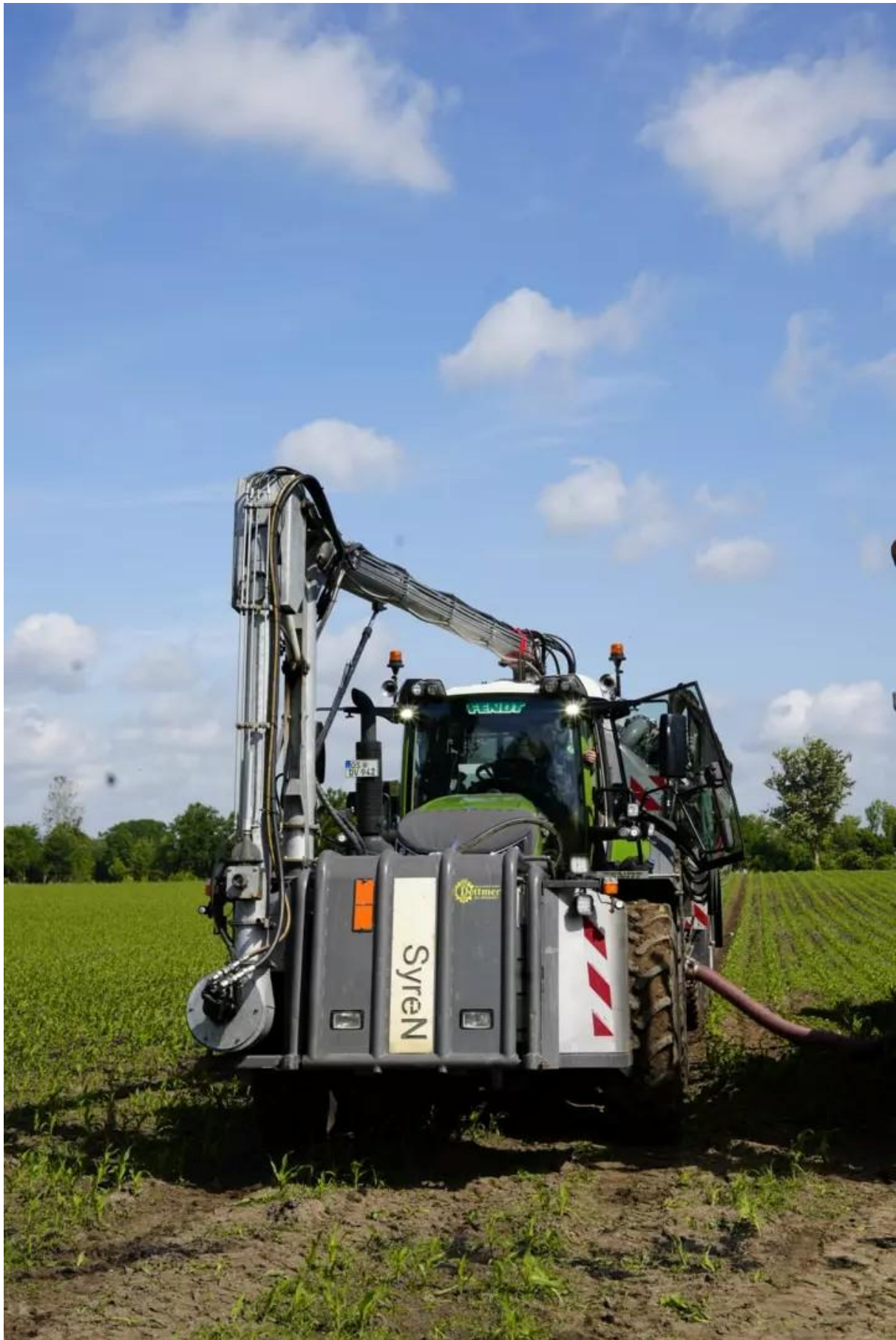
The sulphuric acid container is well protected in the front hydraulics. (Image source: Lillie, Landwirtschaftsverlag GmbH)
