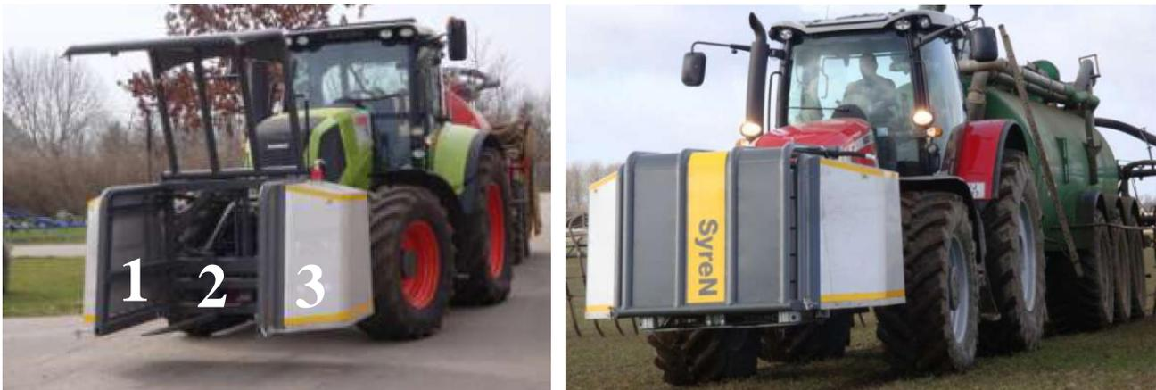
Figure 1. The SyreN-system includes three tanks installed on the front of the tractor. 1: Tank for iron sulphate. 2: Here the tank for sulphuric acid shall be placed. 3: Tank for water for cleaning the system.
