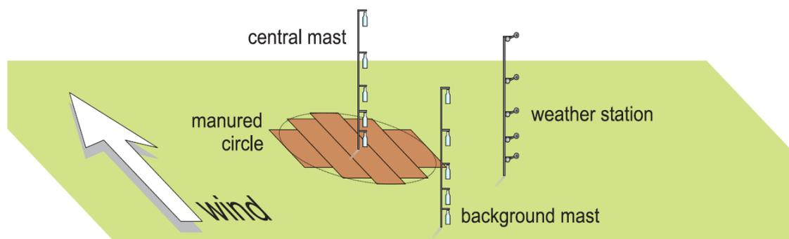
Figure 4. Layout of a circular plot for the measurement of NH<sub>3</sub> volatilization using the micrometeorological mass balance method, with masts supporting NH<sub>3</sub> traps at various heights in the center of the plot and at the windward boundary of the plot. Source: VERA Secretariat, 2009 [2].
