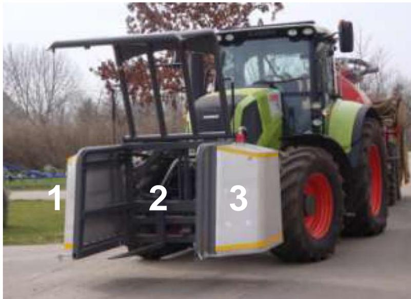
Figure 3. The SyreN-system includes three tanks installed on the front of the tractor. 1: Tank for iron sulphate. 2: Here the tank for sulphuric acid shall be placed. 3: Tank for water for cleaning the system.
