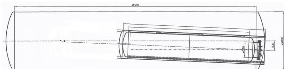
**Figur 1 Ammonia tank integrated in slurry tanker with a side view**
