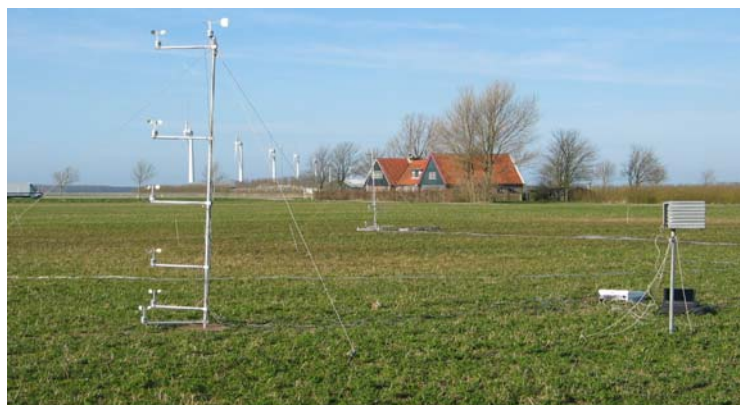
Figure 2. Meteorological mast holding cup anemometers to measure wind speed at five heights. In the background the centrally located mast holding the ammonia traps
