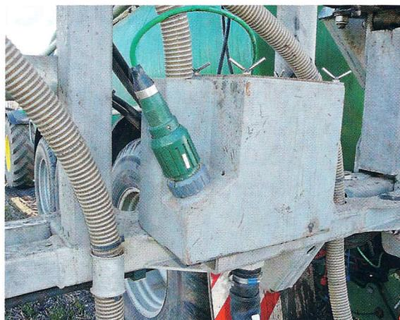
*The applicator-mounted pH sensor determines the amount of acid that needs to be added to achieve the target level.*
