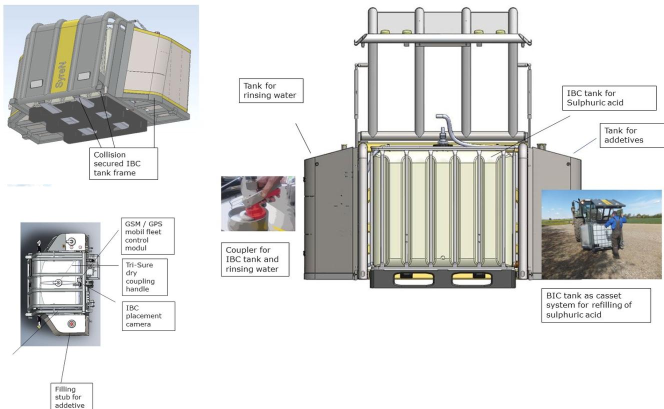
The Front linkage system is constructed with extra safety dimensions and thus is collision-proof. The operating system is an Isobus system and the operation is therefore integrated into the Tractor's own functions such as turn signals, traffic lights and working light. The control is operated through the Tractor's integrated terminal. Alternatively, the SyreN system can use a separate Isobus terminal.
