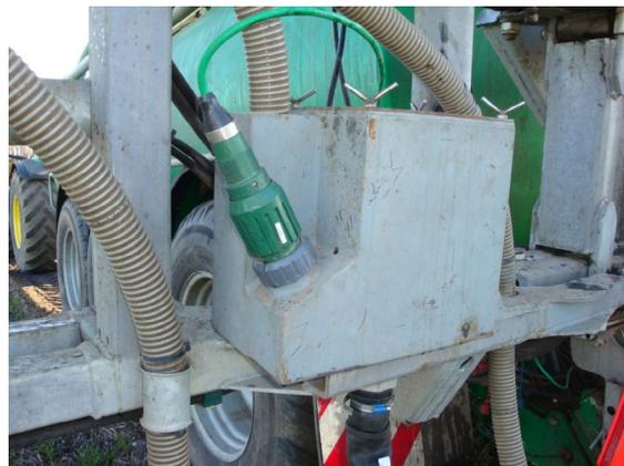
Slurry Sump with PH sensor
