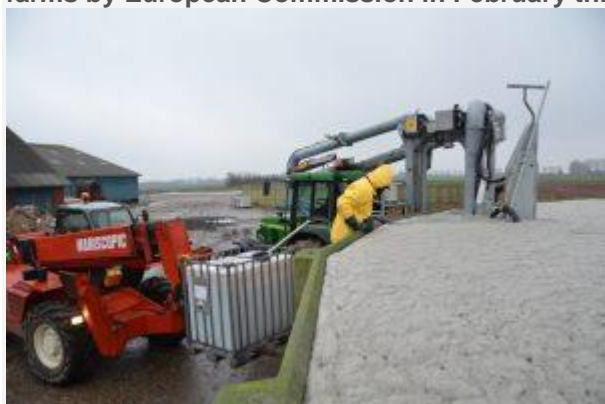
In-storage slurry acidification. Photo: Torkild Birkmose, SEGES.
