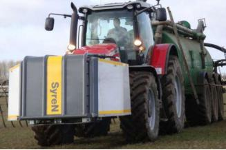
Figure 1. The SyreN-system includes three tanks installed on the front of the tractor. 1: Tank for iron sulphate. 2: Here the tank for sulphuric acid shall be placed. 3: Tank for water for cleaning the system.
