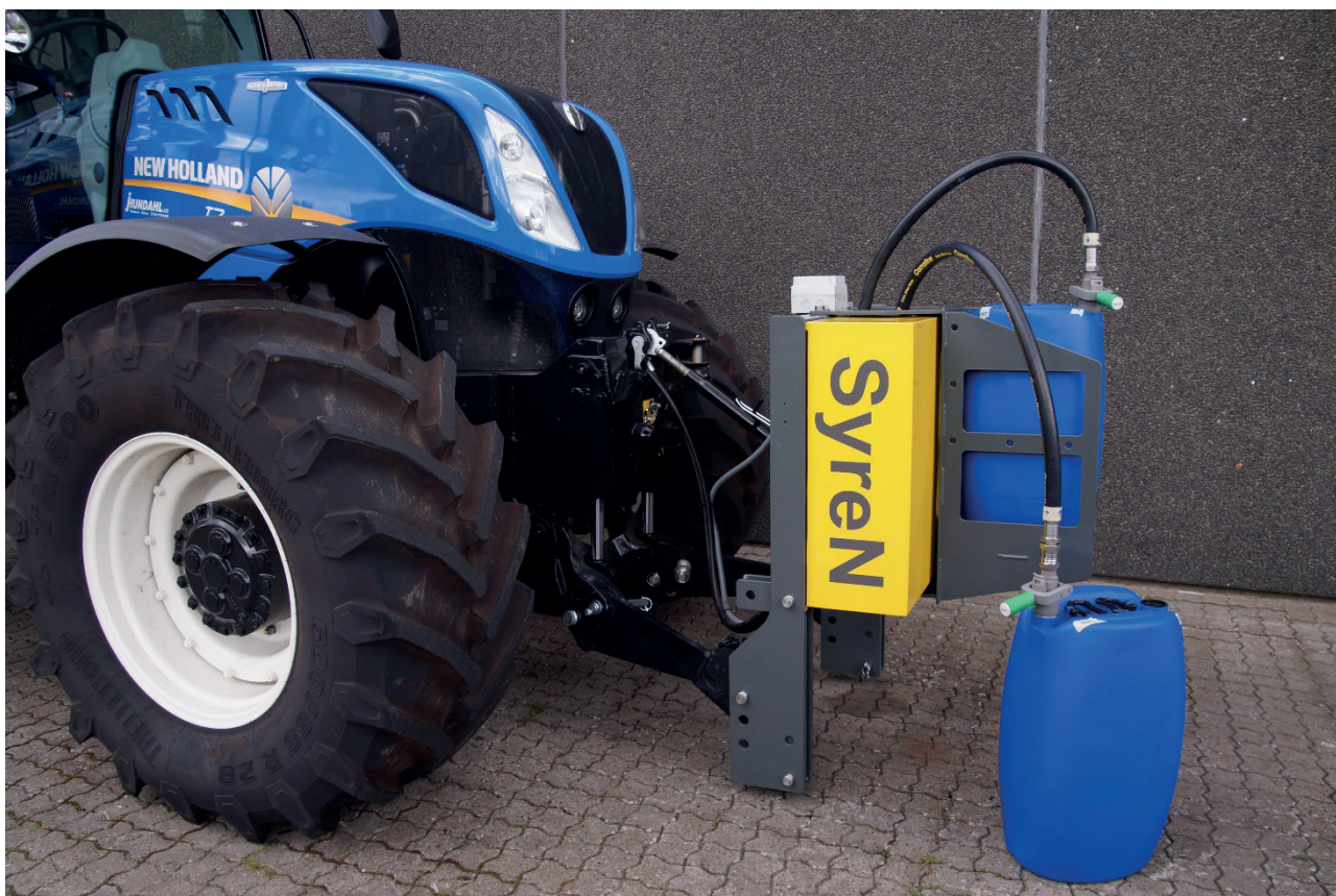
SyreN Light installed in the front hitch
