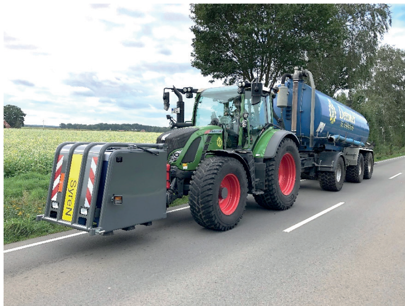
SyreN transporter system with a slurry feeder tanker
