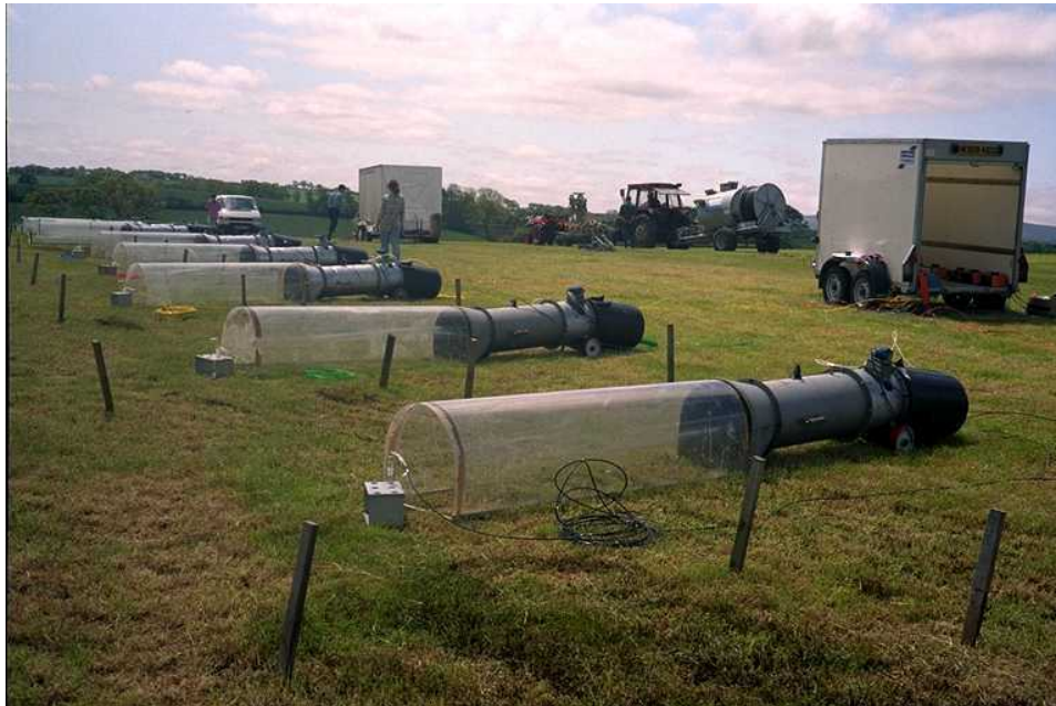
Plate 5.2 Typical wind tunnels used to measure ammonia emissions [Photo: Courtesy of IGER, North Wyke].
