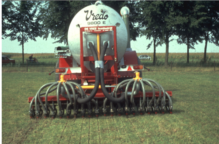
Plate 6.4 Shallow injector. Slurry is placed in shallow slots (5 cm) cut into the soil by using either or both a disc and a coulter. The slots can be left open or closed [Photo: Courtesy of J.F.M. Huijsmans, IMAG].
