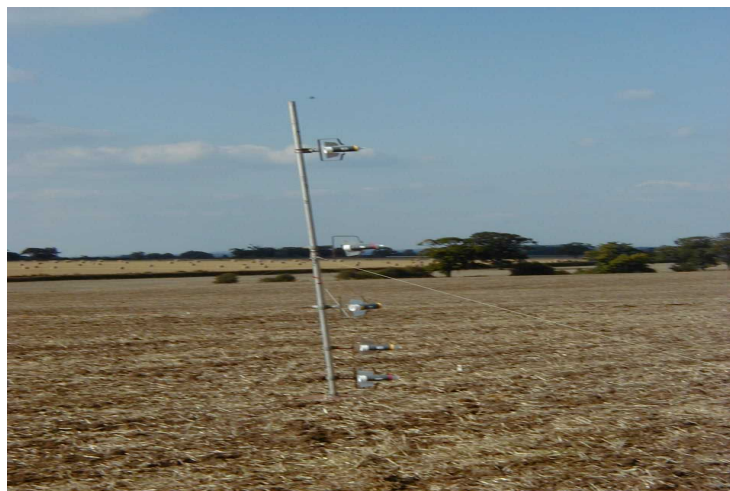
Plate 5.1 The micrometeorological mast used for the measurement of ammonia emissions from field applied manure [Photo Courtesy of IGER, North Wyke].
