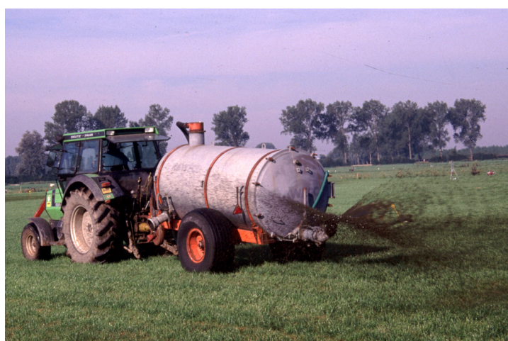
Plate 6.1 Broadcast spreader; still the most common method in most European countries [Photo: Courtesy of J.F.M. Huijsmans, IMAG].
