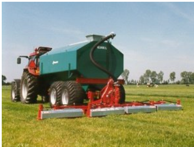
Plate 6.5 The DGI or pressurised injection system [Photo: Courtesy of J. Morken, AUN].
