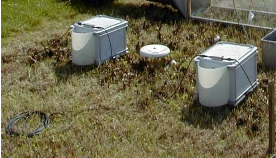
Plate 5.3 The Equilibrium concentration technique, i.e. JTI method [Photo: Courtesy of IGER, North Wyke].
