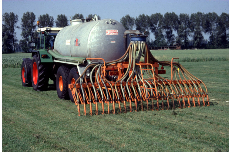
Plate 6.3 Trailing shoe slurry spreader. It places the slurry beneath the canopy thereby reducing the potential for ammonia emission compared with surface applied slurry bands [Photo: Courtesy of J.F.M. Huijsmans, IMAG].
