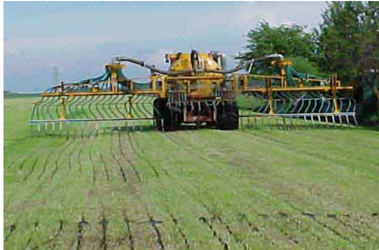
Plate 6.2 Trailing hose slurry spreader. It places the slurry on the soil in bands in the rows between the plants and is particularly suitable for use in tillage crops [Photo: Courtesy of J.F.M. Huijsmans, IMAG].
