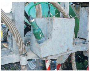
The applicator-mounted pH sensor determines the amount of acid that needs to be added to achieve the target level.
